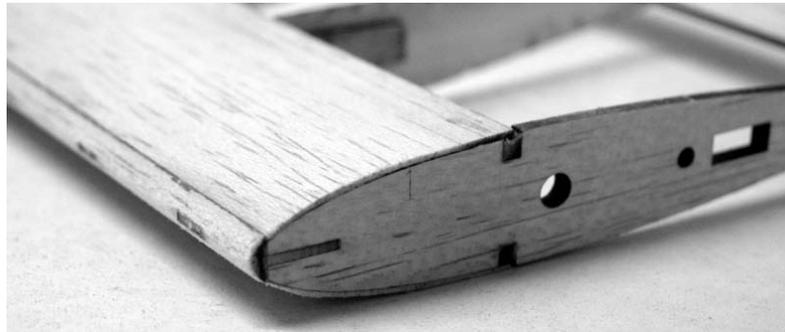
11. Glue the servo tray to the inside of the second rib. The servo tray is on the bottom of the rib and flush with the edge of the rib and spar. Flow some thin CA on the tray to harden the wood so that it will take a servo screw without stripping.
