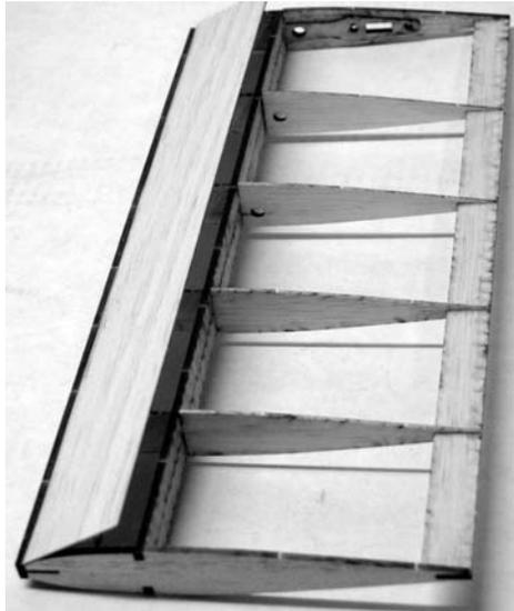
7. Prop the trailing edge up against something flat and level – I use a 3/4" block of wood. When you glue the rear edge of the D Box down, it is imperative that the wing be flat.
