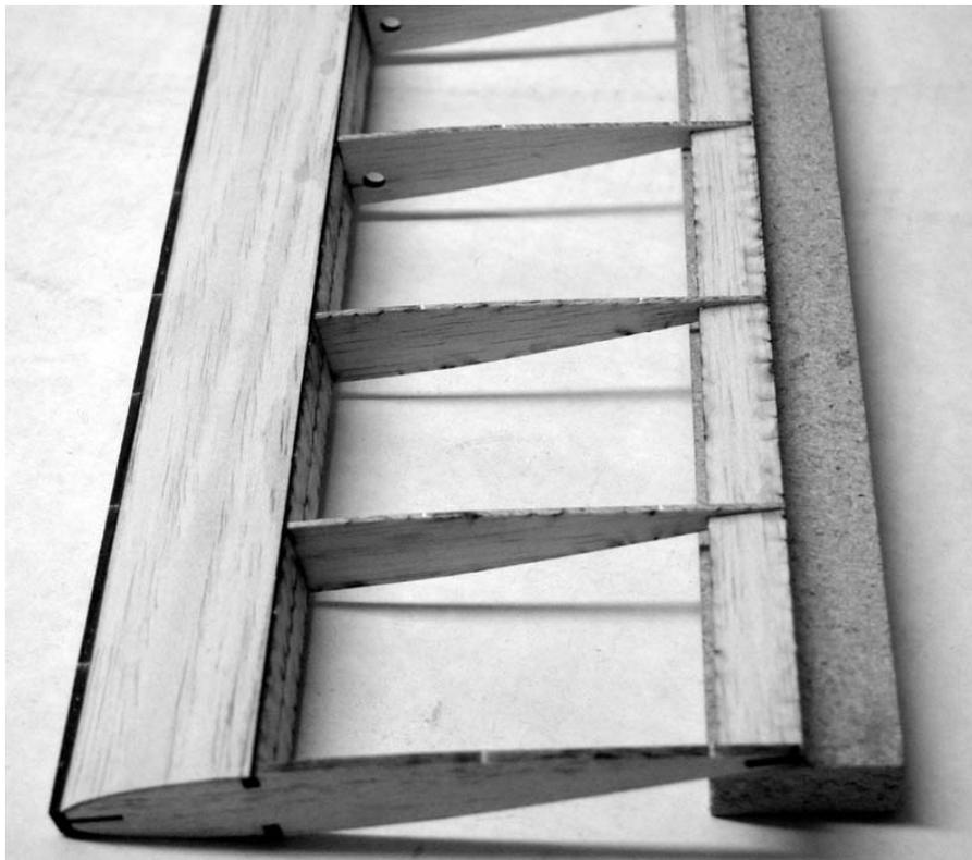
9. Glue the second 1/32" balsa to the other side of the wing. Pay special attention to this side. The wing will not be able to twist once the second side is glued. If you glue this sheet while the wing is twisted, you will not be able to remove it later.
