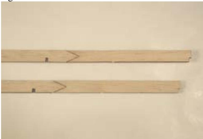
2. Sand the rear edge of the trailing edge to make it rounded.
