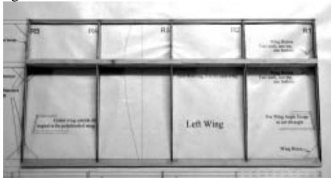
5. Cut trailing edge and lower spar (1/8"x1/4") at the polydihedral break as marked on the plans. This is 14 inches out, or 17.5 inches out for the extended wing. Cut outside the notch on the trailing edge.
