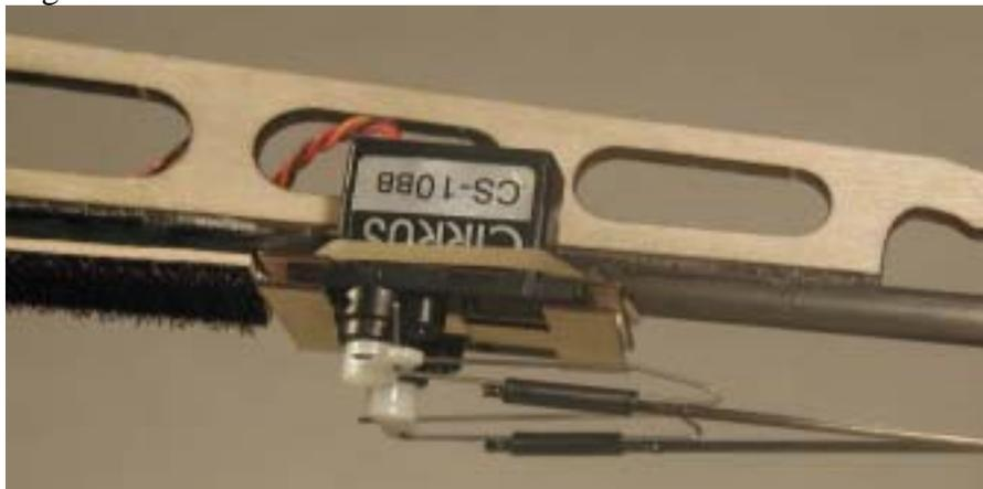
Photo shows underside of fuselage. Note rubber band holding servos in place.
