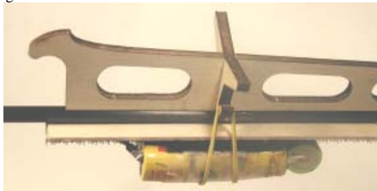
Battery mount showing rubber band backup.
