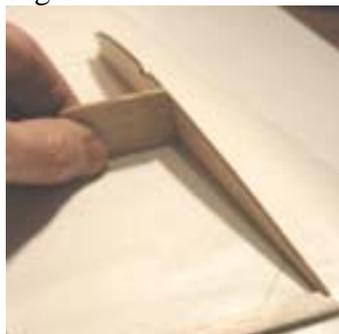
10. Use rib gauge to angle R5 inward (R6 for extended wing) inward.
