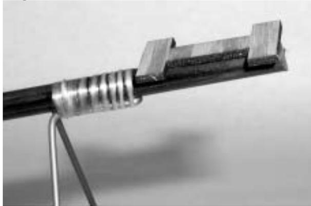
5. Glue wing mount to fuselage with thick CA. Front of wing mount is 3.75" from front of fuselage measured from where the wing mount touches the fuselage. The wing mount should be perpendicular to the work surface when the landing gear is resting on the work surface.
