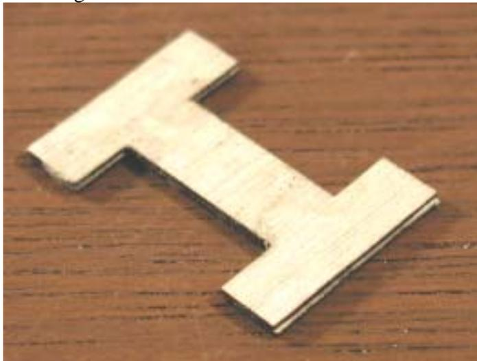
3. Cut out wing mount and wing yoke from 3/32" balsa.
