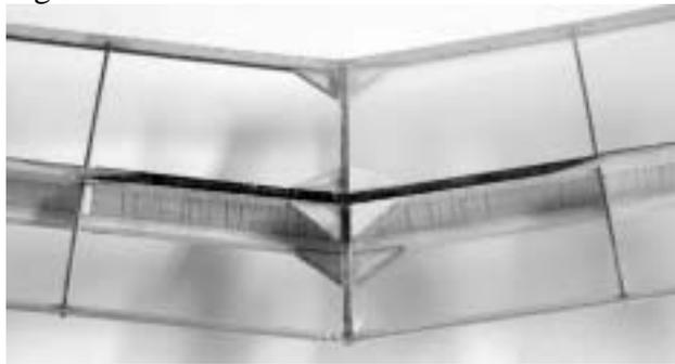
41. To prevent the outer ribs from bowing in when you cover the wings, glue a piece of  $1/8'' \times 1/4''$  balsa from the trailing edge to the spar webbing and another from the spar webbing to the leading edge.
