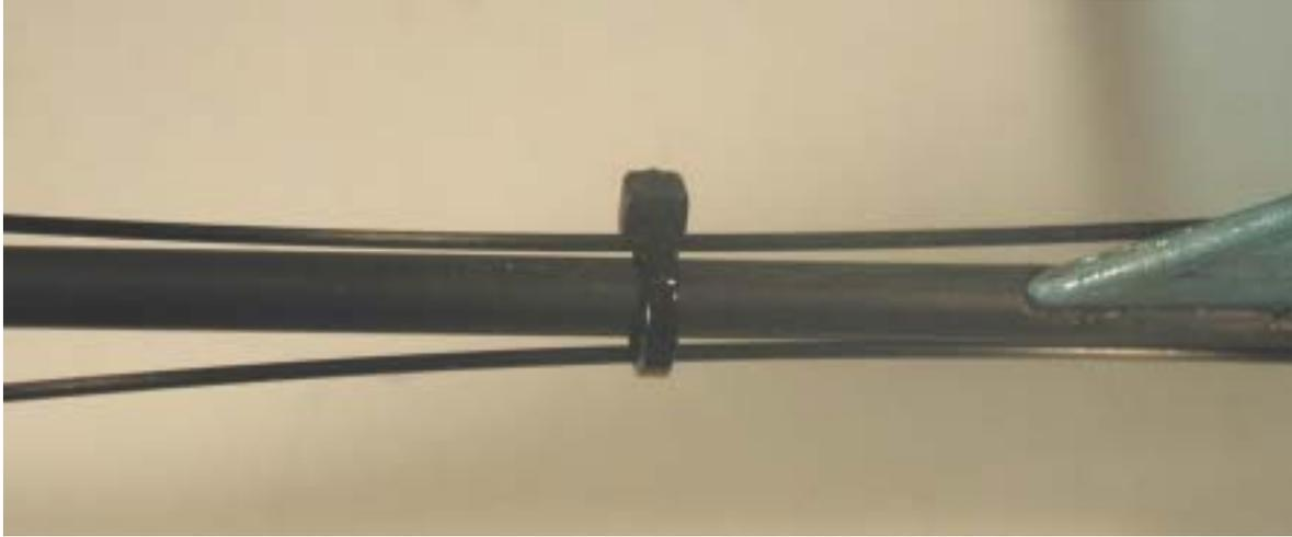
3. Rubber band a 3/16"x5/16" breakaway stick to the motor mount leaving 1 ¼" in front of the mount. Use at least two rubber bands. Slide the GWS motor over the breakaway stick. If it isn't a tight fit, you will shortly have a glider. The breakaway stick has been designed to break before the motor does in the event of a hard landing. Carry extra breakaway sticks with you when you fly.
