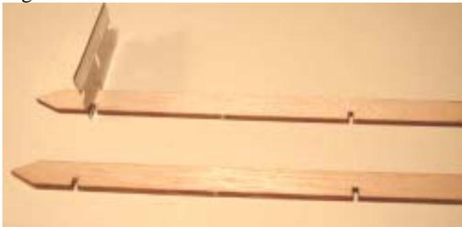
If you are building the extended wing, glue the trailing edge extensions on to the trailing edge pieces with thick CA. Why didn't I just make the trailing edge 25"? The laser cutter will only cut up to 24"!
