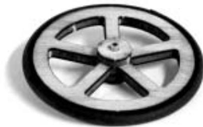
Wrap the tire rubber around your wheel to measure it and cut it 1/16" too short. Glue the ends together with CA. You now have a ring. Slip the ring over the wheel, center it then glue it to the wheel with thin CA.
