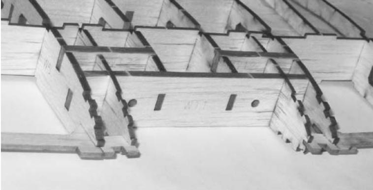
16. With the wing lined up on the plans, glue the trailing edge in place as shown below. Only do one side right now and then we'll do the other side after more is complete.
