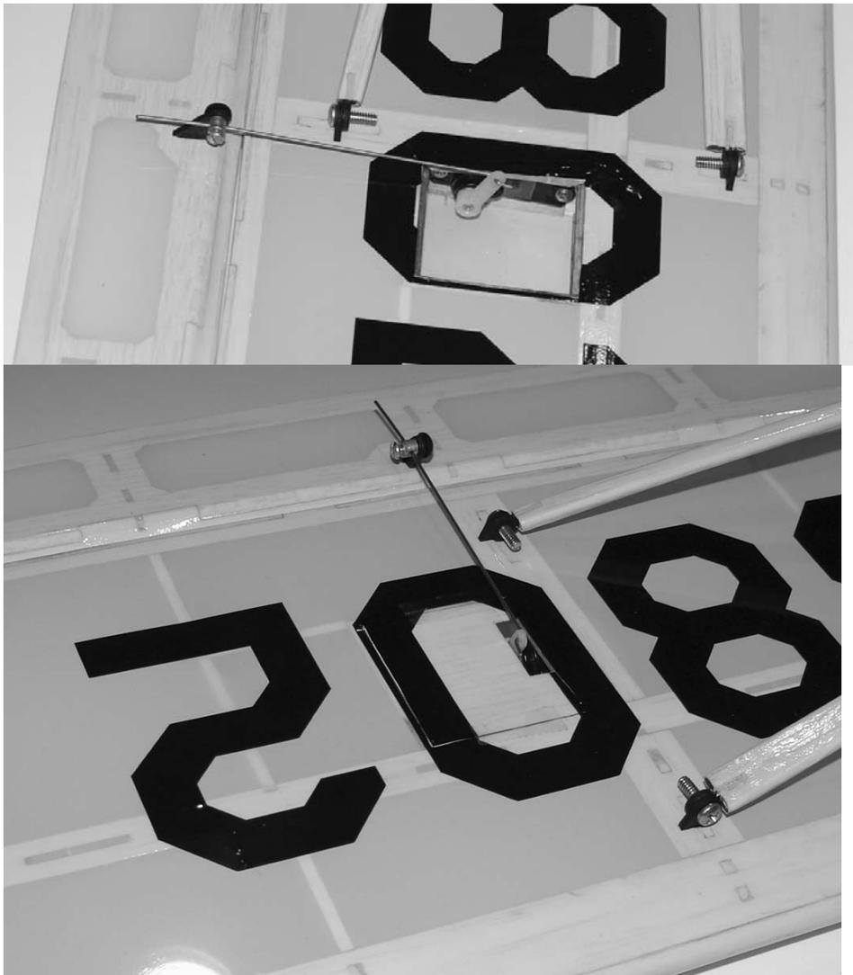
8. Mount the struts as shown in the image above. Once you have threaded the screw, remove it and reinforce the threads in the plywood with thin CA. I have flown my Cubs without the backing nut installed, but do not recommend it. (Do as I say, not as I do kind of a thing!)
