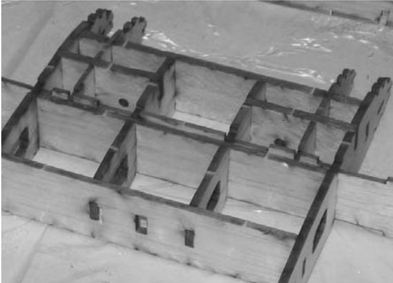
19. With the wing flat and aligned to the plans, go ahead and break out the thin CA. Glue all of the joints. Weighing the wing down to keep it flat helps make sure you don't accidentally warp the wing.
