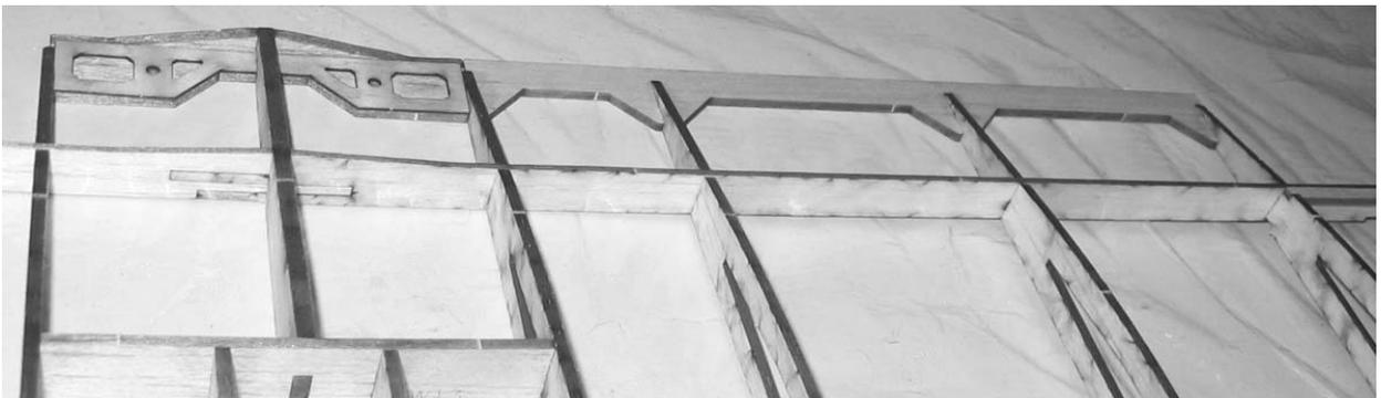
17. Press the 1/8" balsa leading edge into place on the leading edge braces, as shown in the image below. This is on the same wing half as you are already working on, of course. Make sure it is pressed fully in place, but don't glue it yet.
