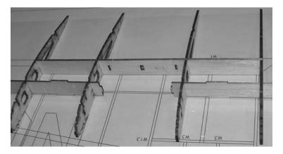
5. Insert the assembly from step 1 as shown in the image below. The W3 ribs tab into W13, the tabs on the ends of the spars go into the W3 ribs, and W11 tabs into the W5 ribs. Do NOT glue anything yet.
