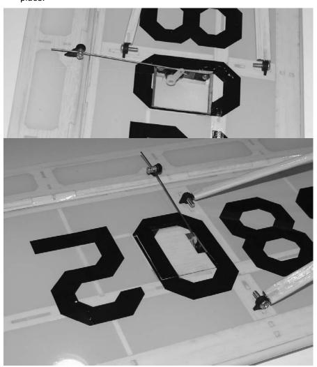
8. **STRUTS ARE NOT OPTIONAL!** Mount the struts as shown in the image above. Once you have threaded the screw, remove it and reinforce the threads in the plywood with thin CA. I have flown my Cubs without the backing nut installed, but do not recommend it. (Do as I say, not as I do kind of a thing!)
