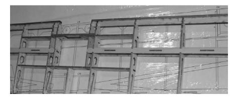
14. Flip the wing over and press the 1/16" top spar "caps" into place, as shown in the image below. The "lasered" side should be facing inside. **BE CAREFUL** where the spar has lightening holes! Put your finger in the lightening hole when you are pressing the spar cap on so it does not break the spar in that area. What happens if you don't do this? You might break the spar of course! So, don't force it. If you need to sand the tabs slightly, do so. Do NOT glue them in yet.
