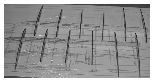
**4.** Press the 3/32" balsa part W13 into the ribs, joining the wing halves, as shown in the image below. Do NOT glue it in yet.
