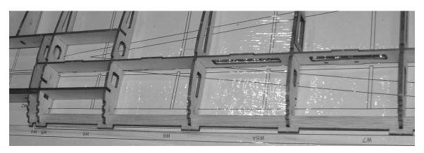
**12.** Press the 1/8" balsa leading edge into place on the leading edge braces, as shown in the image below. This is on the same wing half as you are already working on, of course. Make sure it is pressed fully in place, but don't glue it yet.
