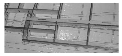
**15.** Install the bottom 1/16" balsa rear spar "caps" and then install the upper rear spar "caps", as shown in the image below. (the uppers plug into W1 at the center of the wing) Guess what??? Do NOT glue them in yet.
