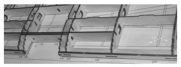
13. Flip the wing over and press the 1/16" bottom spar "caps" into place, as shown in the image below. The "lasered" side should be facing inside. **BE CAREFUL** where the spar has lightening holes! Put your finger in the lightening hole when you are pressing the spar cap on so it does not break the spar in that area. What happens if you don't do this? You might break the spar of course! So, don't force it. If you need to sand the tabs slightly, do so. Do NOT glue them in yet.
