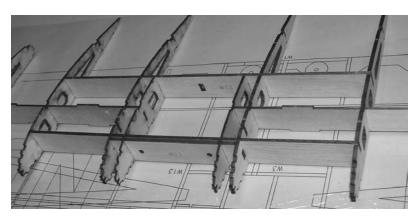
7. Glue the 1/16" rear spar halves together using thin CA. After it has cured, install it by pressing it onto the ribs as shown in the image below. Work a little bit at a time, pressing it into each rib from the inside out just a little bit, then repeat several times, pressing it further into the ribs each time, until it is fully seated in the ribs. Do NOT glue it yet.
