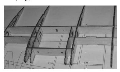
**6.** Test fit the 3/32" balsa W12 part into place as shown in the image below. After you are sure it fits well, remove it and put a very thin layer of 5 minute epoxy on the back of W11 and reinstall W12, making sure everything is straight and F11 and D12 are fully pressed down onto the ribs. Do NOT glue anything else yet. (If you want, you can wick thin CA into the joint after it is assembled instead of using epoxy. We did this on our last wing and it has held up just fine)
