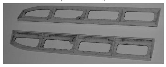
**4.** Assemble the struts over the plans. The "lasered" side of the front part of the strut will match up to the "non-lasered" side of the back part of the strut. Since the laser cuts at a VERY small angle, this makes them match up perfectly and makes the glue joint just a little bit stronger.
