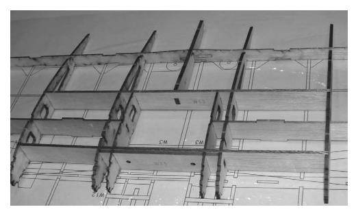
9. Assemble the 3/32" and 1/8" balsa parts for the center trailing edge as shown in the image below. Make sure they are pressed fully into each other, and you finally get to use your CA again to glue them together! Glue the 1/32" ply reinforcing plate to the trailing edge assembly as shown in the image below. Make SURE the bolt holes are lined up. When that's dry, glue the 1/8" balsa doughnuts, making SURE again that the bolt holes are lined up.
