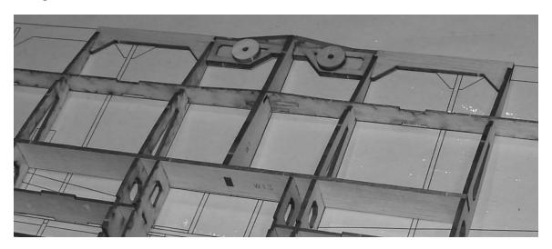
11. Press the long 1/16" leading edge braces into place as shown in the image below. Press them in a little at a time into each rib like you did with the rear spar. Do NOT glue them in yet.
