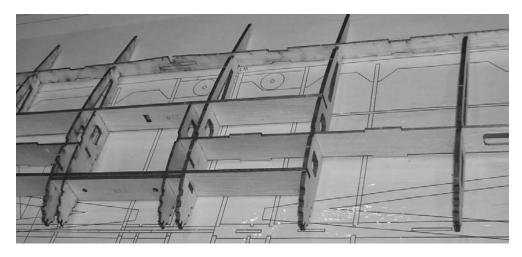
8. Press the tab on the 1/8" W1 part into W13 and slide it into the slot in the rear spar. Do NOT glue it yet.
